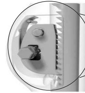
A miniature ratchet mechanism allows the elongation of an expandable rod
